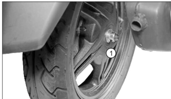
3. Slightly tilt the vehicle and take out the wheel from the rear axle.
