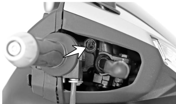
3. If the brake fluid level is below the mark or while applying brake if you feel the brake is more spongy or ineffective due to air entry, contact TVS Motor Company Authorised Distributor or Dealer / Authorised Service Center for topping-up the brake fluid, air bleeding and other brake related inspections.
