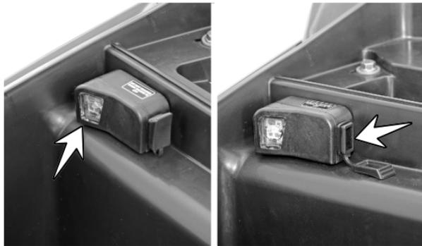
4. Do make sure the flap is not damaged while opening / inserting the USB cable.
