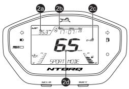
To enter into sport mode, short press the 'Mode' button in street mode while 'Trip B' in display. In sport mode, the following features will be displayed
