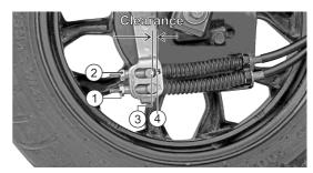
6. After adjusting the adjuster nut top, If any clearance is observed in between the bullet bottom (5) and the slot bottom (6) marked as "I" as shown, then turn the adjuster nut (2) in anti-clockwise until there is no clearance.
