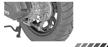
7. Replace the fibre washer while reassembling the oil level screw
