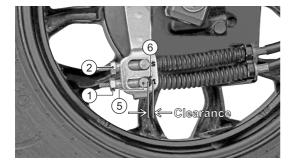
Since the vehicle is fitted with Synchronised Braking System (SBS) adjust the brakes with additional care. If not it may result in brakes not working properly. Please contact TVS Motor Company Authorised Distributor or Dealer / Authorised Service Center for any further assistance.
