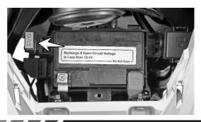
Turn 'ON' the ignition lock and check for proper functioning of the electrical systems. Incase the fuse fails again, consult the nearest TVS Motor Company Authorised Distributor or Dealer / Authorised Service Center.
