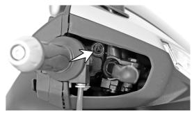
3 If the brake fluid level is below the mark or while applying brake if you feel the brake is more spongy or ineffective due to air entry, contact TVS Motor Company Authorised Distributor or Dealer / Authorised Service Center for topping-up the brake fluid, air bleeding and other brake related inspections.
