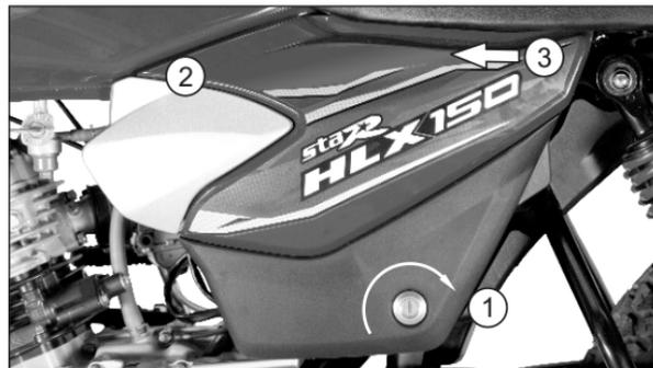
1. Insert the key in the cover frame at lock (1) and rotate it in clockwise direction.
