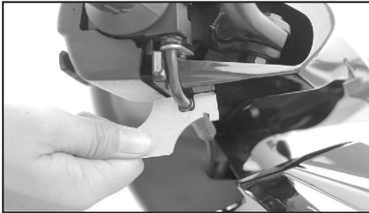
Open end to adjust throttle cable play.
