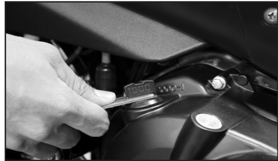
Open end to open & tighten dipstick oil.
