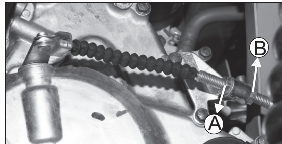
Clutch cable adjustment
