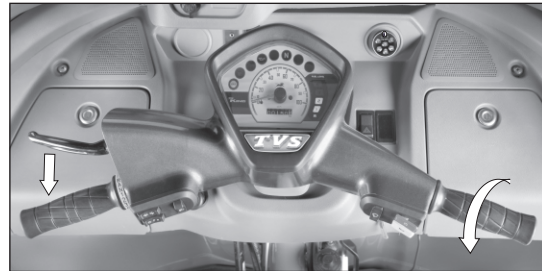
Setting the vehicle in motion
