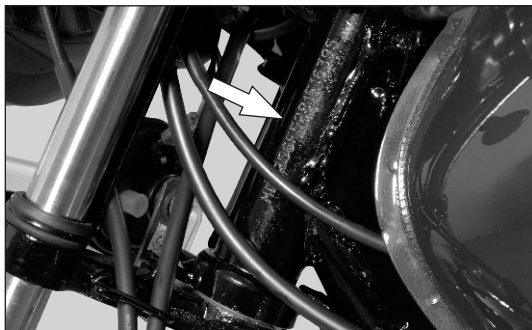
The frame serial number is stamped on the left side of the steering head tube.
