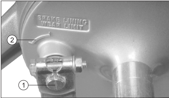
Brake wear indicator mark
