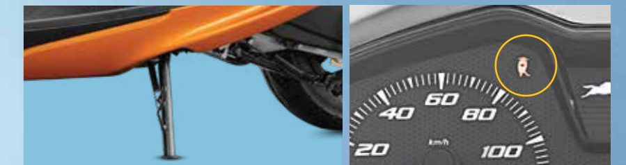
SIDE STAND INDICATOR & INHIBITOR This safety feature ensures that the engine cuts off when the side stand is engaged, improving rider safety
